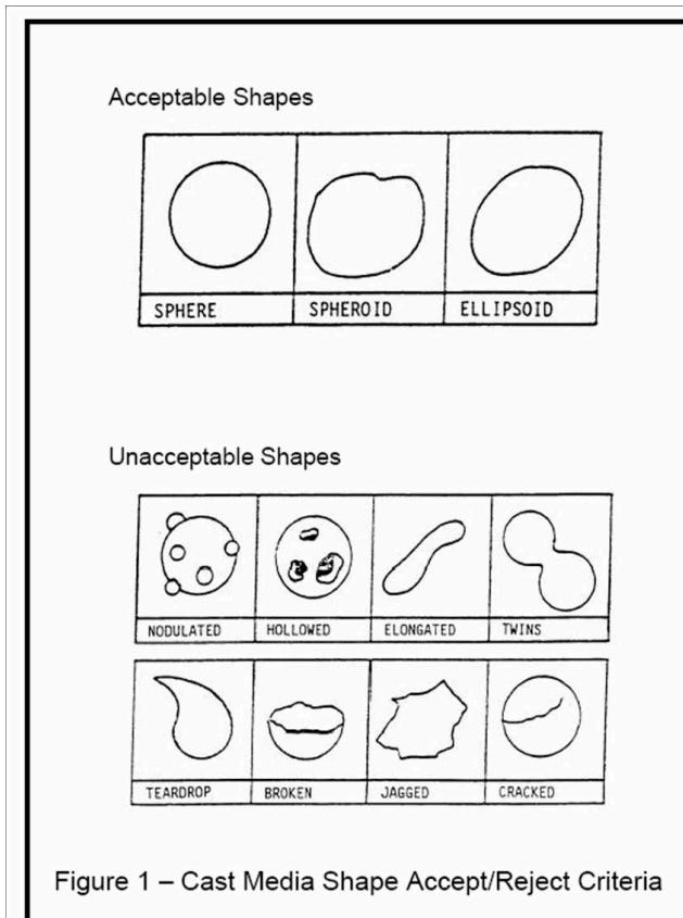
Figure 1 – Cast Media Shape Accept/Reject Criteria
