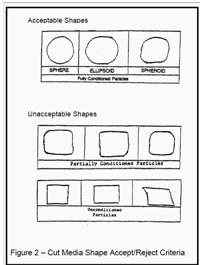
Figure 2 – Cut Media Shape Accept/Reject Criteria
